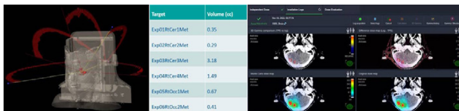
Fig. 1: A six-target SRS case using a single isocenter. It's planned with one coplanar arc and three non-coplanar arcs. The target volumes ranged from 0.29 cc to 3.18 cc (left). As compared with the treatment planning dose, myQA iON's Monte Carlo dose calculations based on log-file data yielded a gamma passing rate of 99.95% using a passing criterion of 3%/1mm with a 10% dose threshold (right).
